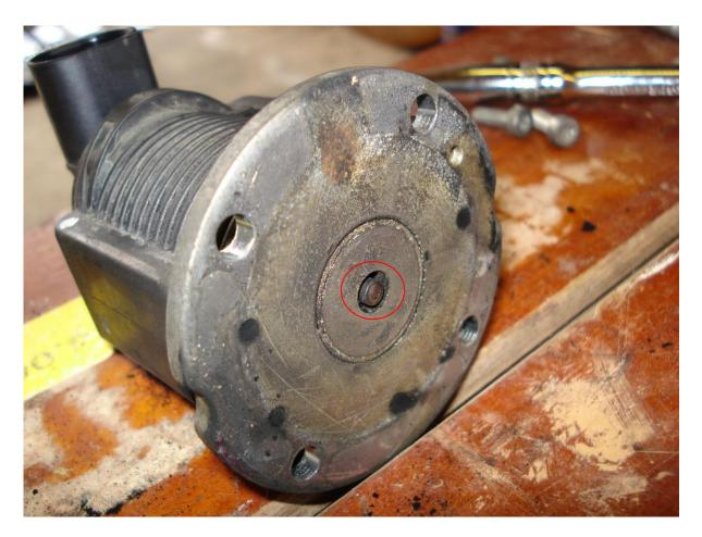
Securely hold the EGR solenoid in a vice or work bench. Drill a hole 3mm to 4mm in diameter in the plastic as shown in the picture. Next take a 3mm or 4mm punch to the inside of the solenoid, and knock out the insides. If might take quite a bit of force... be brave... and catch the insides when they come out !
