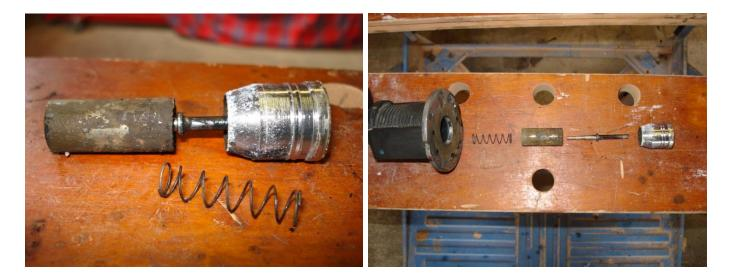
Clean up all parts of the solenoid, with a little wet 'n' dry paper or similar. Clean out the inside of the solenoid casing. Smear, the solenoid with grease, I used Ceratec, but I'm sure it doesn't make a huge difference, although I'd shy away from copper slip, it obviously not ferrous, so will not be affected by the electromagnet but, all the same..
