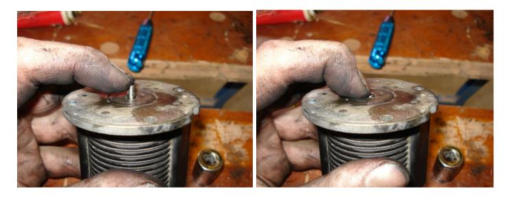
Dry out the EGR body that has been soaking in Carb Cleaner, and re-attached to the Solenoid. Remember the mark you made earlier? Align the marks.
