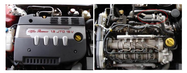
The EGR valve is located on the inlet manifold at the rear right of the engine.
