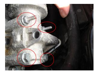
Next, remove the four bolts holding the EGR to the inlet manifold (4 x 10mm, 2 will require a spanner or long reach sockets). Two are regular bolts, two have short stubs for the oil breather pipe bracket.
