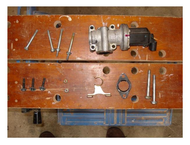
Next step is to remove the EGR solenoid from the EGR valve body, it's held on with 4 x T25 Torx bolts.
