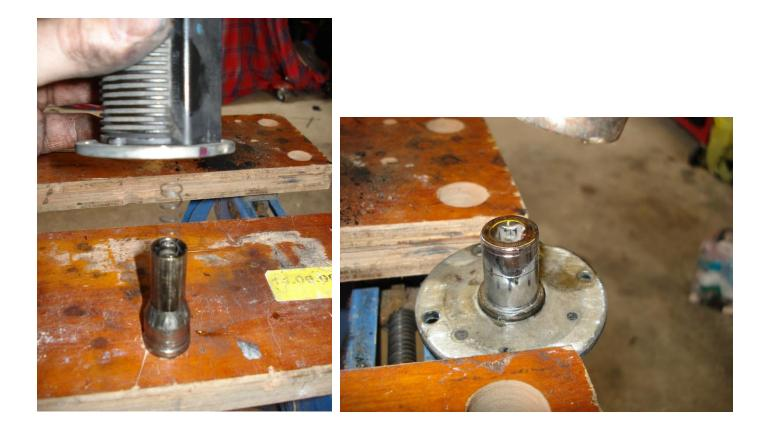
Once it's all back in place, the pin on the solenoids internals should easily be able to move in and out, it should be sprung to the out position. If you can't push it in and out with minimal effort, a little more cleaning may be required.
